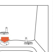
5. Put the cap into the hinge base. Fix the seat cover into the hinge base. Finish.
