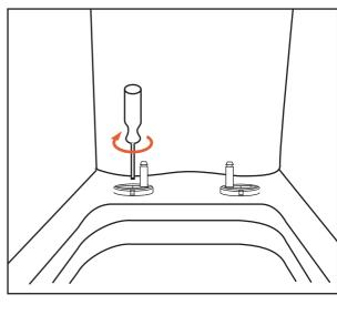
4 Lock the support completely on the ceramics and cover with stainless steel cover.
