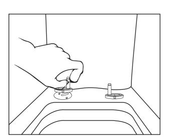
Insert the screw on the hinge base into the holes on the pan.
