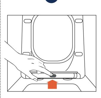
6. Press the button down and pull up to easily remove the cover plate for convenience. Clean.
