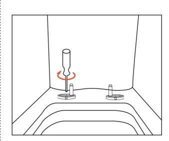
2. Tighten the setscrew but not to the end in order to adjust the seat cover properly.
