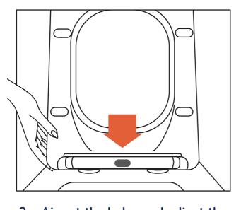
3. Aim at the holes and adjust the hinge base to make the seat cover and pan match.
