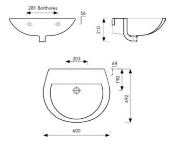
The Atlas Medical Basins with 2-piece Concealed Stability Brackets Combo comprise a medical wallmounted basin, as well as a 2-piece, powder-coated Concealed Stability Bracket set.
